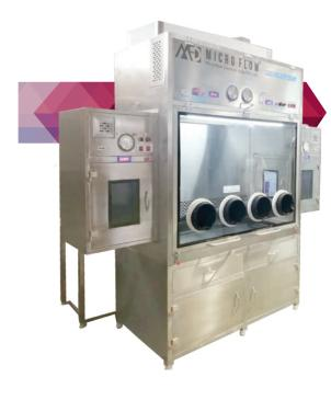
**CLASS III CABINETS** are defined as a totally enclosed ventilated unit of gas-light construction. Operations in the cabinet are conducted through hand-holes with rubber gloves. The cabinet unit is maintained under negative air pressure of at least 0.5 inch water gauge (12.7mm WG).
